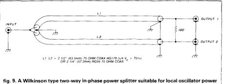
fig. 9. A Wilkinson type two-way in-phase power splitter suitable for local oscillator power splitting in the range of 800-900 MHz. Other frequencies can be used by adjusting the length of the 75 ohm coax for 0.25 electrical wavelength at the desired frequency.
